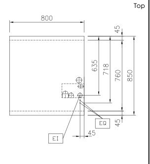
Electric Supply voltage: 400 V/3N ph/50/60 Hz Electrical power max: 12 kW **Key Information:** 100 °C **Working Temperature MIN:** Working Temperature MAX: 450 °C External dimensions, Width: 800 mm External dimensions, Depth: 850 mm External dimensions, Height: 250 mm Net weight: 120 kg Configuration: One-Side Operated;Top Front Plates Power: 3 - 3 kW **Back Plates Power:** 3 - 3 kW Solid top usable surface 670 mm (width): Solid top usable surface
